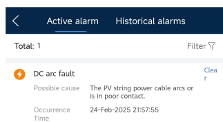
Figure 7-7 Clearing the alarm
