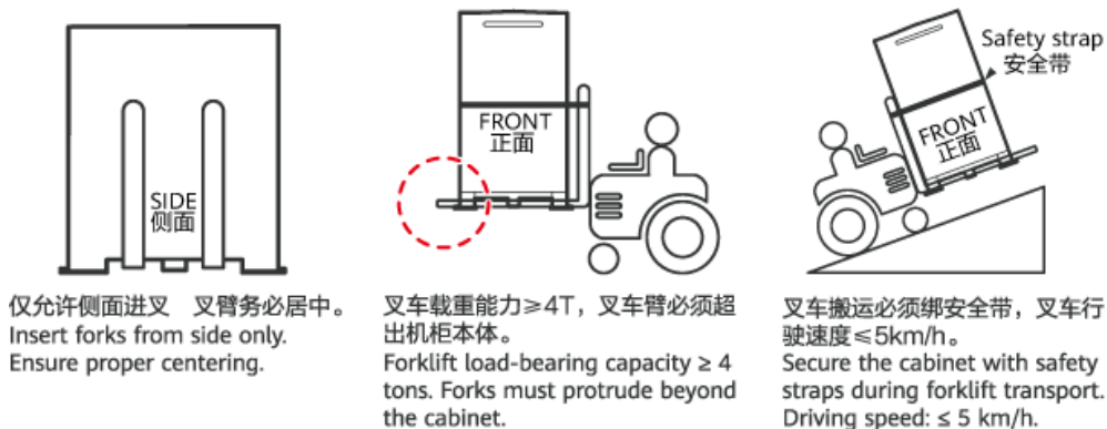
Figure 3-1 Loading and unloading requirements
