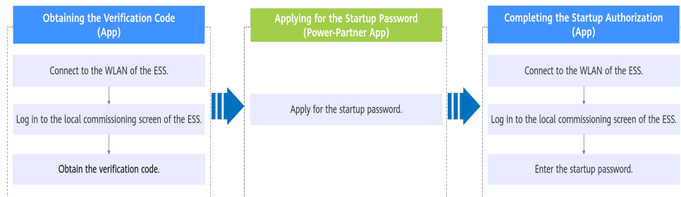
Figure 9-2 ESS startup authorization procedure
