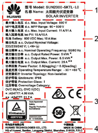
Figure 2-9 Nameplate of the SUN2000-5KTL-L0
