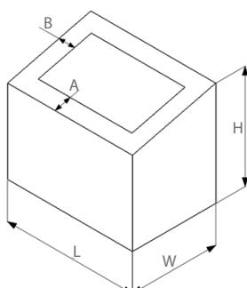
Indication of zones with increased suction forces of the wind is determined on the basis of general dimensions of the building (Fig.1), where:
